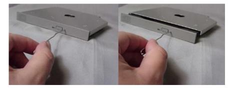
Figure 2.Using Emergency Eject
